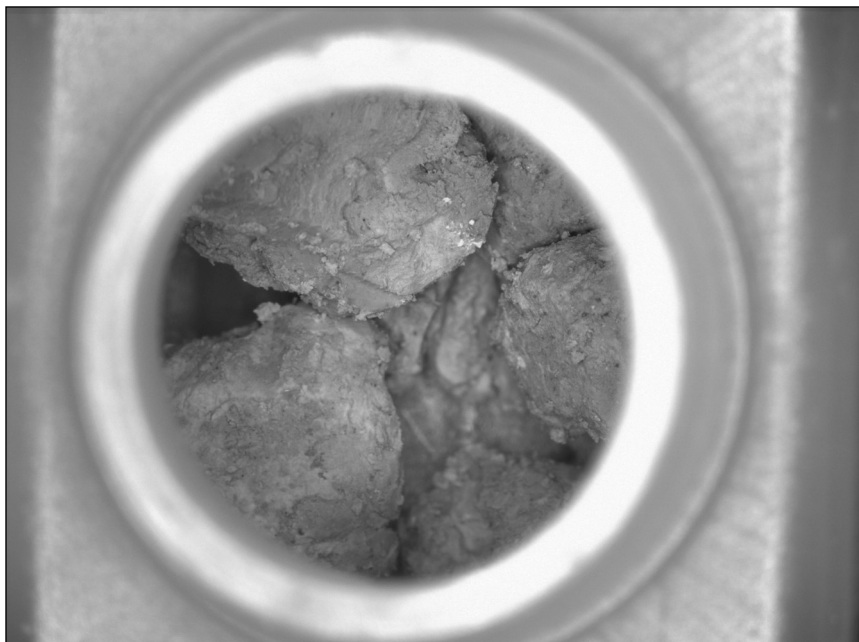
Figure 3.1. Sample of uranium ore concentrate seized at Rotterdam in 2003, after arrival at the nuclear forensics laboratory
