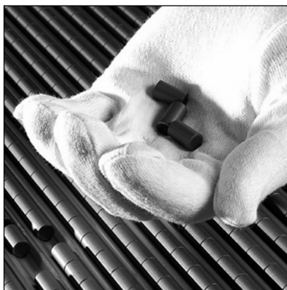
Figure 5.4. Examples of uranium oxide pellets used in nuclear power reactors
